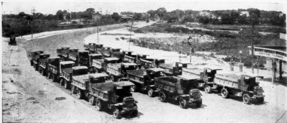
These Autocar trucks are equipped with Heil steel dump bodies 10' 6" long, 6' 6" tapered in width, 27" high. No. 5 Heil Hydro Hoists are installed on the entire fleet.
